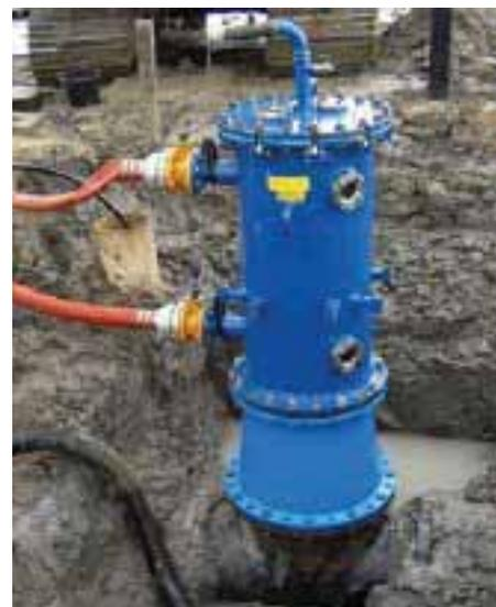
Left: Mobile flow measurement at inspection endpoint
